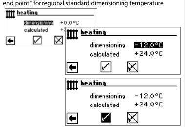
The program of the heating and heat pump regulator now calculates the actual return temperature at -12 °C for the heating curve end point and displays this in the menu field "Calculated". In the example+24,0 °C:
