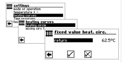
If the option "Fixed temperature" is switched on by the system setting, the screen changes to the menu "Heating curves" (which can take you to the menus "Fixed value heating circle" or "Fixed value mixing circle") or directly to the menu "Fixed value heating circle".
