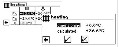
Menu line "dimensioning" Menu line "calculated" regional standard design temperature Calculated temperature heating curve
