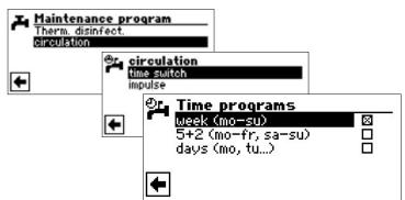
Use the time programs to specify the times during which the circulation pump is to run.
